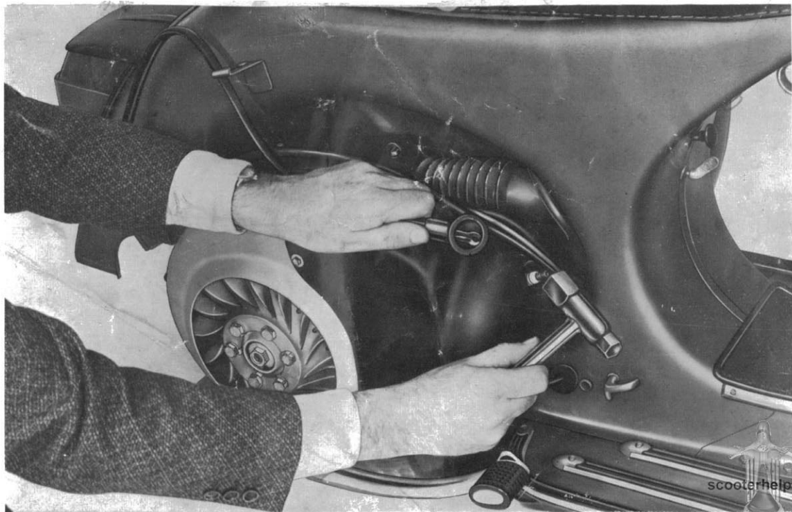
Fig. 15 - Dismantling spark plug
